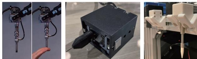
Fig. 7 Different tool types. Left: Screw tool with suction and compliance. Middle: Screw tool with compliance and without suction. Right: Passive tools.
