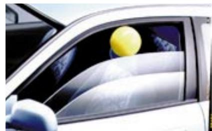
*This power window switch has an antipinching function to prevent it from closing on arms or other obstacles. When an obstacle is encountered, the switch causes the window to stop and reverse in motion.*
