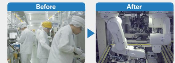
Fully automated robots suspended from the ceiling install parts in devices and move parts between processes, tasks which formerly required 10 workers.
