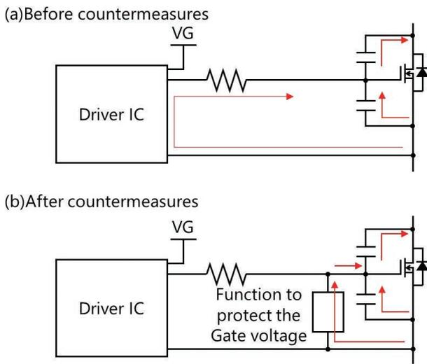
Fig. 5 Function to Protect the Gate Voltage
