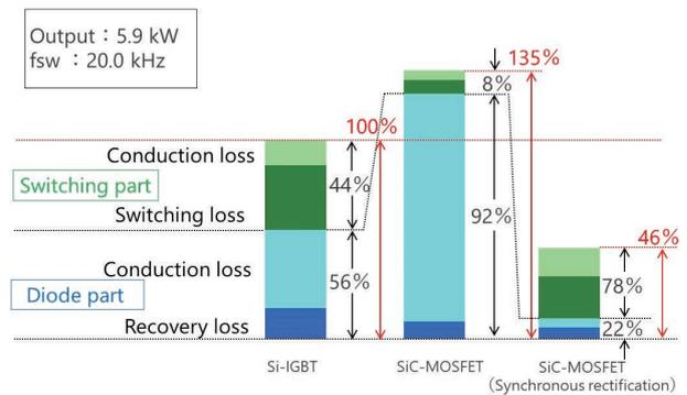
Fig. 7 Effect of synchronous rectification
