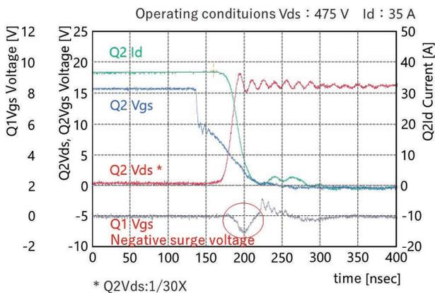
Fig. 6 Gate Voltage waveform
