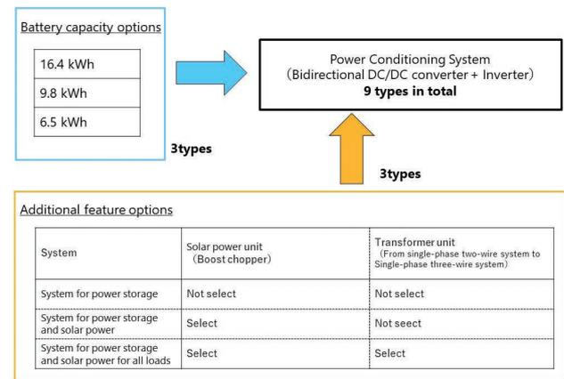
Fig. 1 Options for System Configuration
