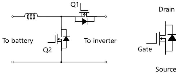
Fig. 4 Non-insulation Type Bidirectional DC/DC Converter and SiC-MOSFET
