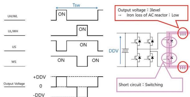
Fig. 10 System Devised for Reducing Loss
