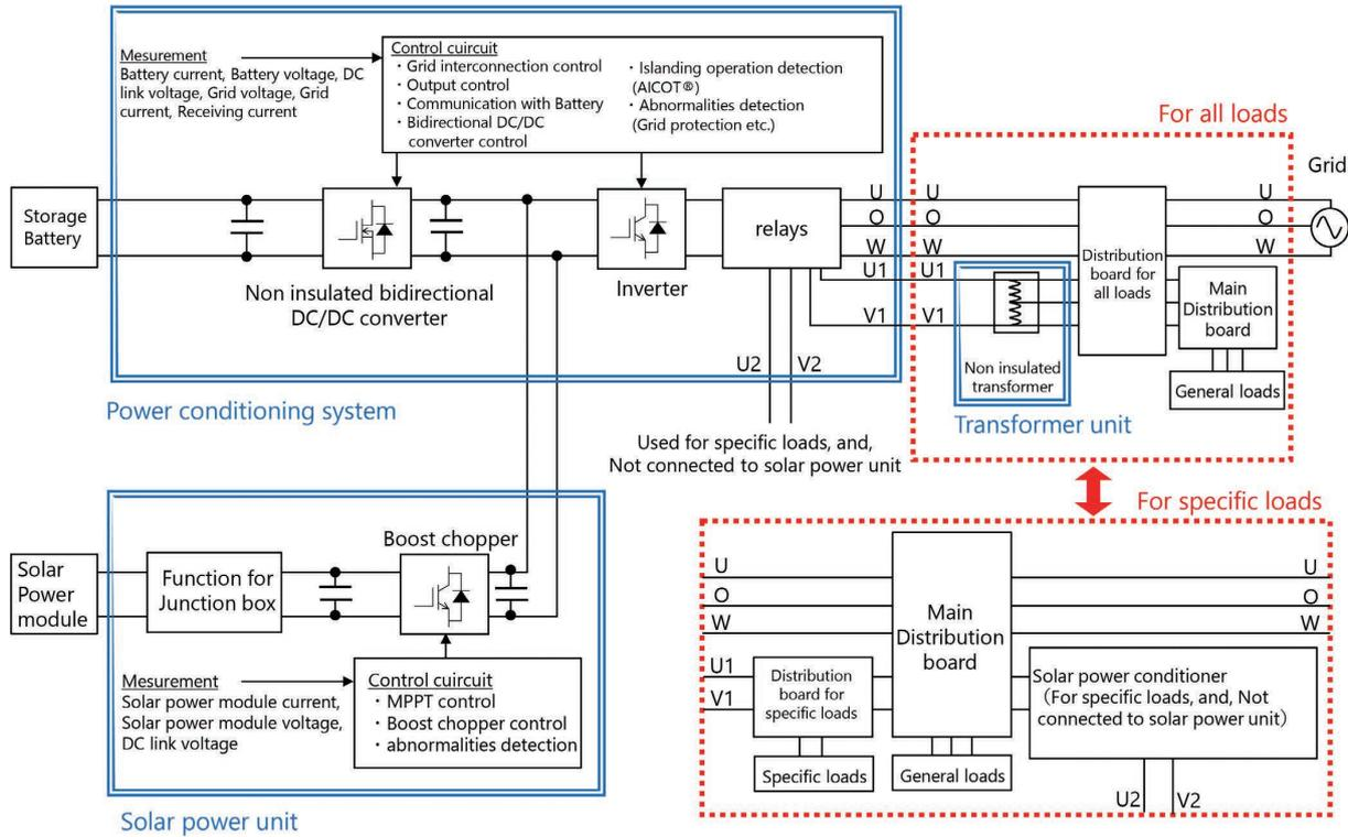
Fig. 3 Circuit Structure of KPBP-A Series
