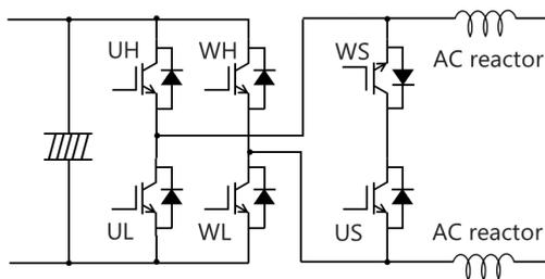
Fig. 8 Circuit Structure of Inverter Part
