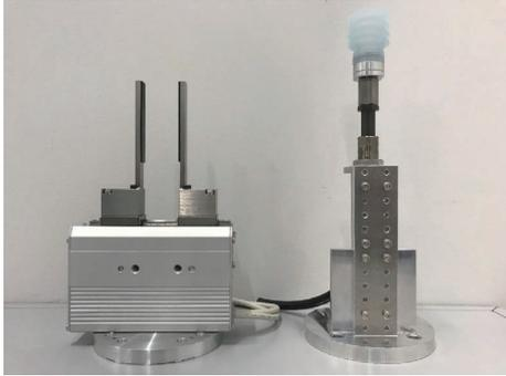
Fig. 1 Two-fingered hand (left) and suction hand (right)
