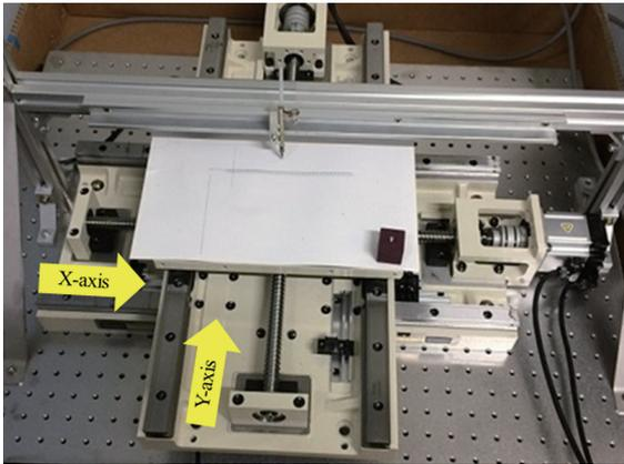
Fig. 4 X-Y stage used for test
