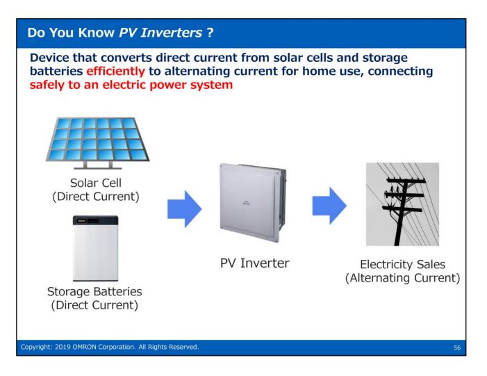
• The function of a PV inverter is to efficiently convert direct current from PV panels or storage batteries so it can be safely used in the home, enabling safe connectivity to the power grid.
