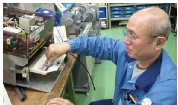
Developer modifying a standard automatic sealer for use by an employee with disabled hands
