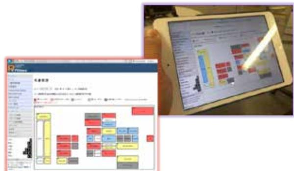
Total visibility on one screen. See production line information at a glance. Red line indicates production line delays.
