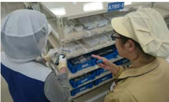
Omron Taiyo introduced barcode readers for more efficient part picking
