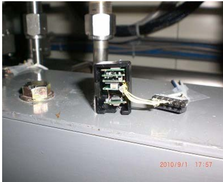
Acoustic sensor on a pump
