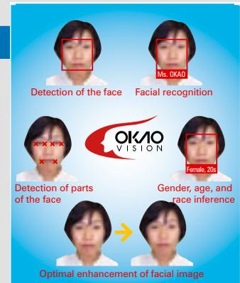
\* Facial image enhancement functions: Functions to enhance skin color and so forth at the time of printing by the detection of a “face” from an image obtained by a digital camera, etc.
