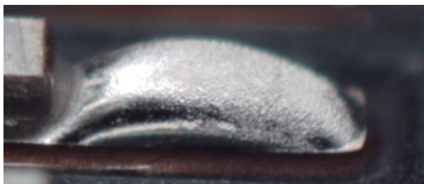
Fig. 3 Shape of non-wetted solder (external view)
