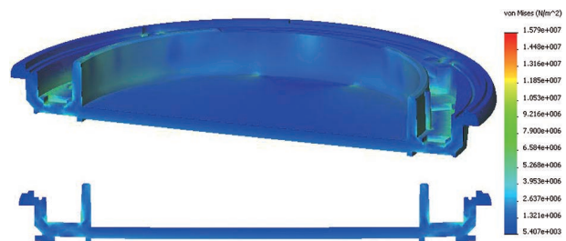
Fig. 10 Stress analysis results of button attachment part
