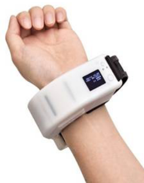
Fig. 12 The prototype continuous sphygmomanometer we developed
