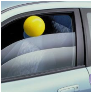
This power window switch has an antipinching function to prevent the window from closing on arms or other obstacles. When an obstacle is encountered, the switch causes the window to stop and reverse automatically.
