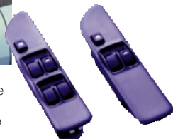
This power window switch has an antipinching function to prevent the window from closing on arms or other obstacles. When an obstacle is encountered, the switch causes the window to stop and reverse automatically.
