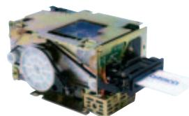
Applicable in ATMs, financial services kiosk and other networks. This next generation of card reader/writer incorporates the needs of both contact and Contact-Less IC cards, and is able to fit various IC card standards by modifying the program.
