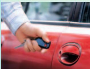
This system is to lock or unlock doors by remote control in conjunction with hazard lamp. The maximum distance between transmitter and receiver is expanding, and the sensitivity of the sensor is increasing.
