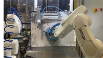
Two OMRON robots shaping blue polyurethane circle parts
