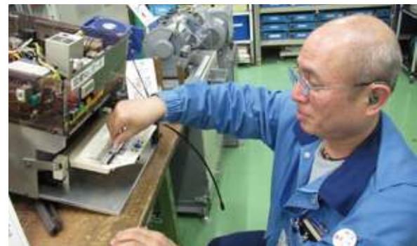
Developer modifying a standard automatic sealer for use by an employee with disabled hands
