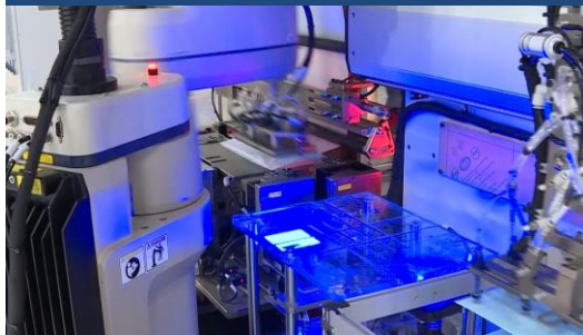
Process where electrode positioned by robot is wrapped in laminate film (Demo machine at Automation Center in China)
